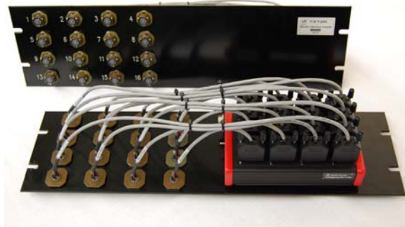
Custom designed Bendix Interface Adapter panel based on a Titan Input Module
