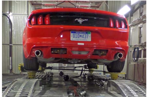
A Ford Mustang on a four-poster tire-coupled road simulator
