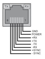
The Titan CPU08V has eight identical Titan Input Module Port connectors. LEDs integrated into these connectors indicate when a connected Titan Input Module is transmitting and receiving data. Titan Input Modules connect to these ports using industry-standard 'straight-through' Ethernet cabling, which provides power, sync and data connections on a single cable. The maximum recommended cable length from the Titan CPU08V to a Titan Input Module is 25'.
